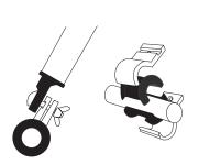
6. Lift the top horizontal tube and mount the T-connector to the top horizontal tube and the telescopic leg.
